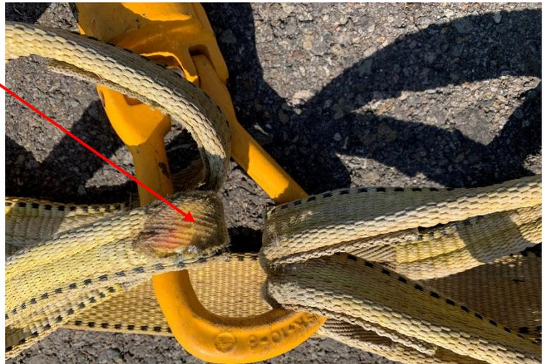
Faded areas, showing UV damage to straps
