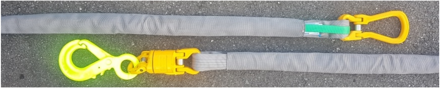
Fig.: The absolute classic among tactical lines. A striking feature in this combination is the lemon-yellow OBK safety hook: Gunnebo Industries started their range with grade 8 products compliant with EN 1677, but then began replacing and amplifying their assortment piece by piece with grade 10 products.
