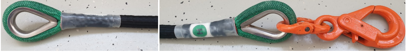
Fig.: Special-design line with flame-retarding sheathing and position marking.
