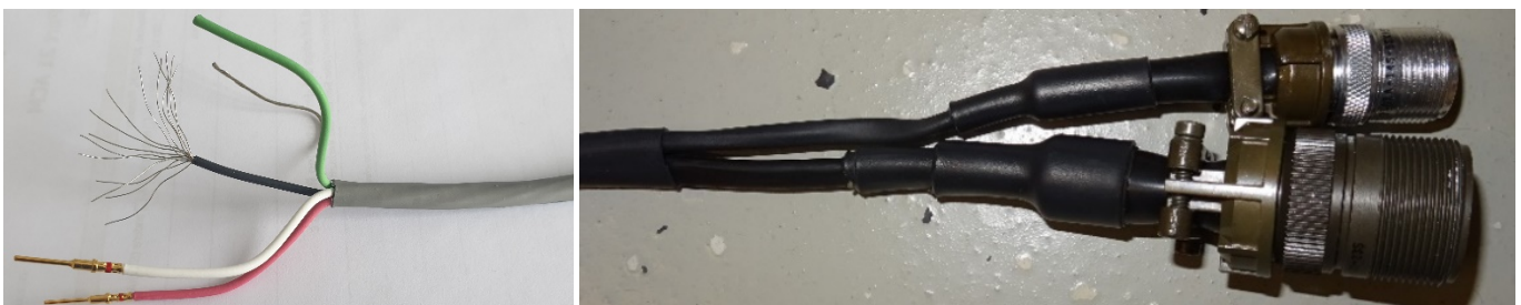
Fig.: 4 x AWG18 electric conductor including a ground wire ( A = 0.823 \text{ mm}^2 ) and crimped pins
