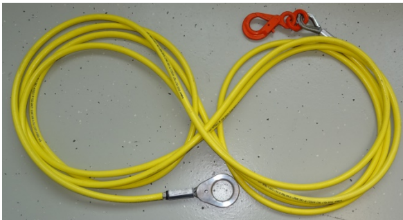
Fig. TLSS steel line with yellow protective sheathing. Steel lines must be flaked in a figure of eight (to distribute the tension), then folded up to a ring.
