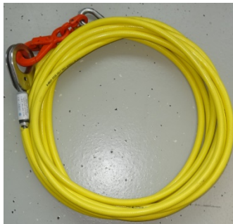
Fig. TLSS steel line with yellow protective sheathing. Steel lines must be flaked in a figure of eight (to distribute the tension), then folded up to a ring.
