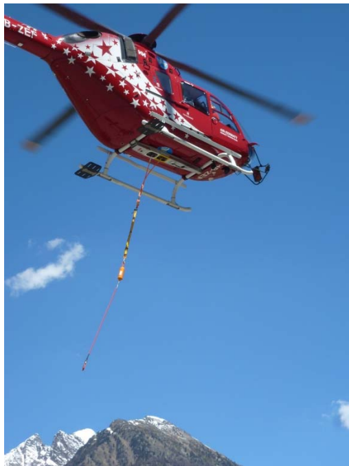
Fig. 1: Shortest rope length (5.7 m), without payload. Y-rope, shock absorber and weight element.
