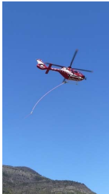
Fig. 2: 15.7 m at 65 kts, i.e. 10 m of rope extension.
